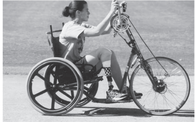
Figure 29-7 Independent or group activity: hand-crank three-wheeled bicycle.
