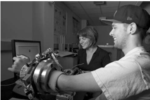
Figure 18-1 The Rice Robot, a fully articulated exoskeleton for spinal cord injury (SCI) rehabilitation, mimics upper extremity joints from shoulder to hand. (Courtesy of the Mechatronics and Haptic Interfaces Lab, Department of Mechanical Engineering & Materials Science, Rice University, Houston, TX.)
