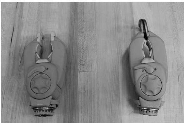
Figure 41-8 Ottobock (Minneapolis, MN) Greifer terminal device. The Greifer on the left has the interchangeable standard hooks and is in open position. The Greifer on the right has interchangeable extended hooks and is in the closed position.
