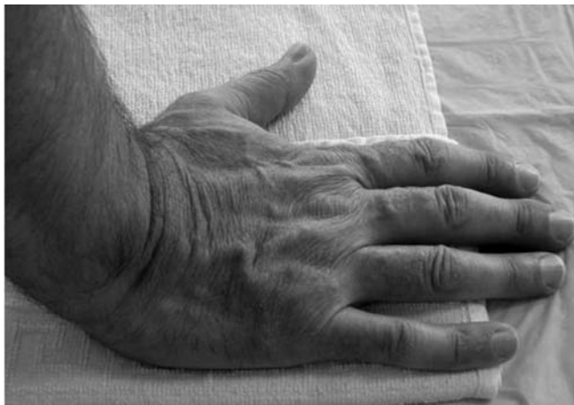
Figure 16-24 Pressing into heated plastic with a cotton towel removes the material laminent, which prepares it for self-bonding.
