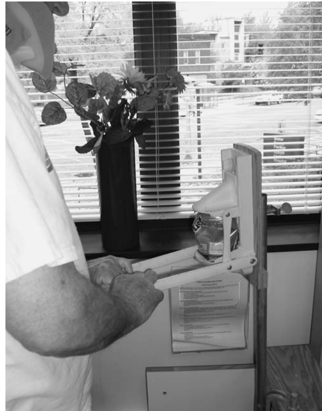
Figure 12-8 A patient who has weak upper extremities is able to crush cans for recycling because the handle (force arm) of the crusher has been elongated.
