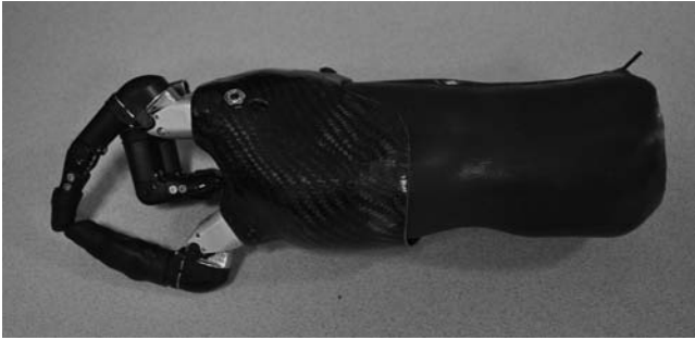
Figure 41-31 An example of a final prosthesis for an individual with a partial hand amputation using ProDigits™ by Touch Bionics, Inc. (Hilliard, OH).
