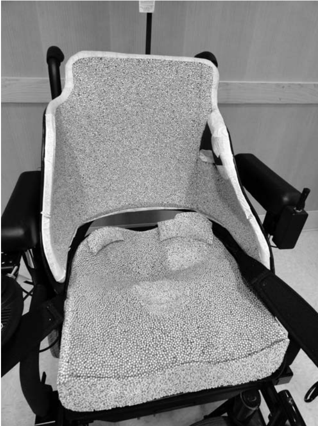
Figure 17-5 Custom contouring. Specialty manufacturers make custom cushions and backrests from a direct cast molding of the individual, through an electronic sensing system or by foam-in-place methods. These systems are typically used with individuals whose unique postural needs cannot be well supported by premade cushions or backrests.
