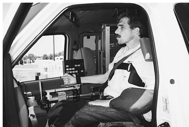
Figure 26-27 A high-technology driving system to assist a person with quadriplegia to operate the controls of a van while sitting in his wheelchair. (Courtesy of Driving Systems Inc., Van Nuys, CA.)
