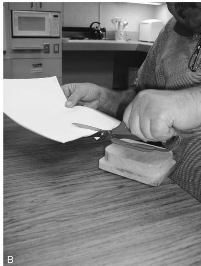
Figure 12-5 A, B. Scissors have been stabilized in a wooden block to enable cutting by a person who lacks finger dexterity.
