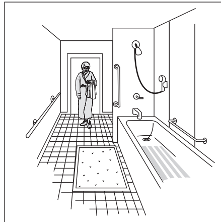
A vertical grab bar provides support when entering the tub, while an horizontal (or angled) bar helps you to complete the entrance and lower yourself onto a shower seat or to the bottom of the tub.
