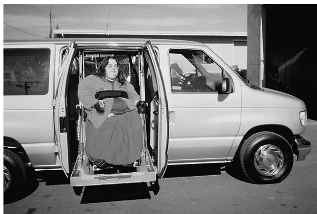
FIGURE 11-25 A platform-style lift can be located at the side or rear of a van. Additional entry headroom, obtained through a lowered floor, provides client with appropriate visibility when driving from a power wheelchair.
