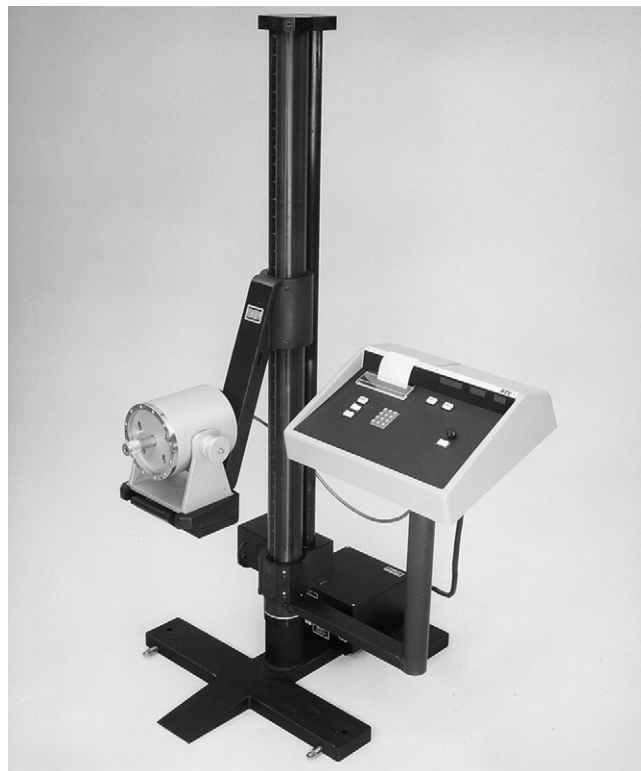
FIGURE 39-18 BTE Work Simulator is an electromechanical device used to simulate real-life tasks for upper extremity evaluation and strengthening. The client's progress is monitored through a computerized printout, and the program can be modified to increase resistance and endurance.
