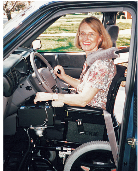
FIGURE 11-19 This client was experiencing difficulties driving and at work, as progression of her multiple sclerosis exceeded the activity demands of pushing a manual wheelchair. Driving from a power wheelchair and using an electronic gas-brake hand control decreased the activity demands on her upper extremities, enabling her to drive safely and work full-time as a teacher.
