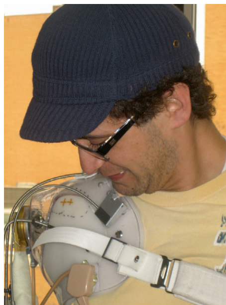
FIGURE 43-16 Nudge control used to operate the elbow unit for shoulder disarticulation prosthesis.
