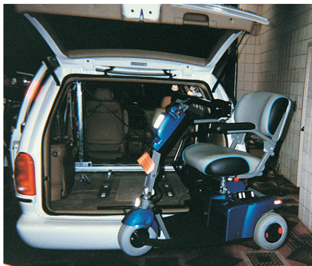
FIGURE 11-24 The Curbsider, by Bruno, hoists a scooter or a fully assembled power wheelchair, up to 250 lb, from the sidewalk and lifts it into the back of a standard minivan.
