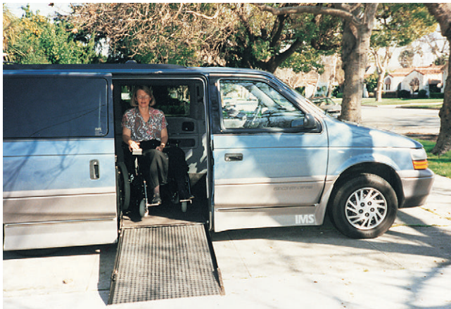
FIGURE 11-26 Minivan conversion with side ramp access and a lowered 10-inch floor. The ramp angle can be decreased for easier entry and exit.
