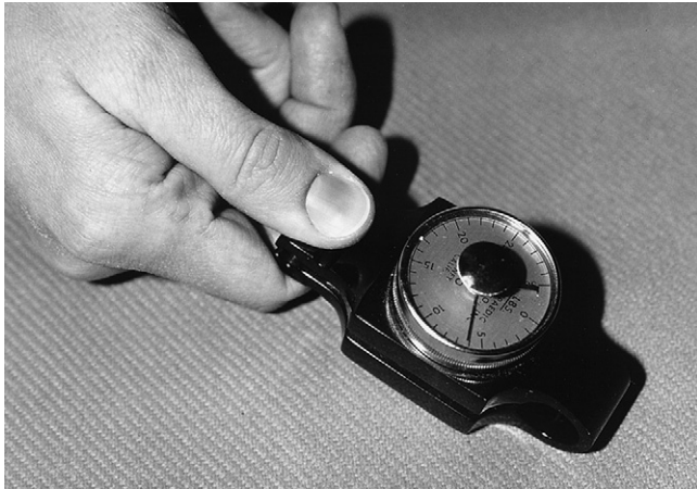
FIGURE 39-3 Pinch gauge is used to evaluate pinch strength to a variety of prehension patterns of pinch.
