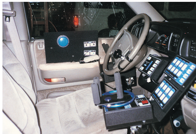
FIGURE 11-22 High-tech equipment compensates for limited motor skills. The evaluation van equipped with electronic mobility controls (EMC) has a left-side electronic gas-brake, a remote left elbow secondary control button, a 7-inch remote steering wheel ( on right ) with trip-in steering device, and a membrane switch console for functions including gear shift, windows, and headlights.
