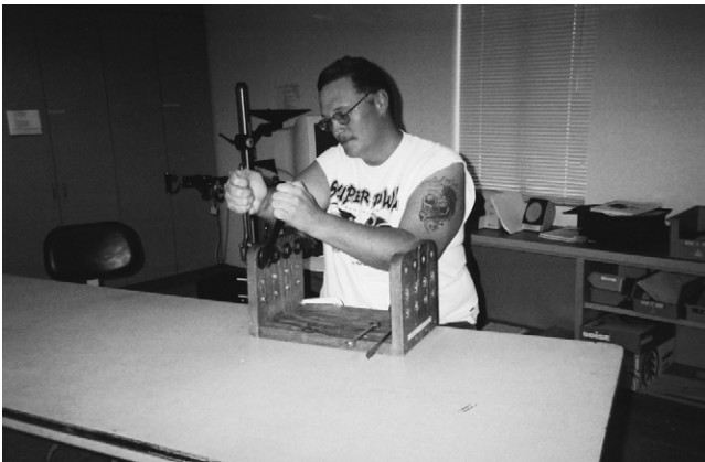
FIGURE 14-4 The Bennett Hand Tool is a dexterity test to assess a person's ability to use hand tools.
