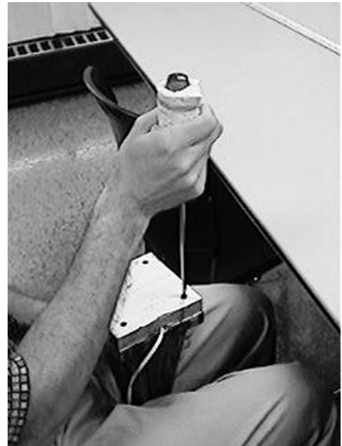
FIGURE 29-6 The size of tool handles may be increased by padding the handle with foam rubber.
