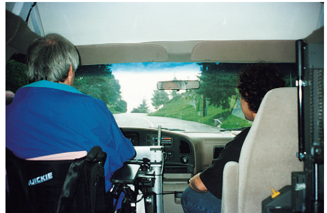
FIGURE 11-29 This client drives a steep mountain pass near his home. During the follow-up evaluation in his new Driving Systems, Inc. (DSI) unilver van, a test drive was performed in nearby foothills to ensure that adjustments were adequate for steep inclines. This essential step identified additional adjustments needed before delivery.
