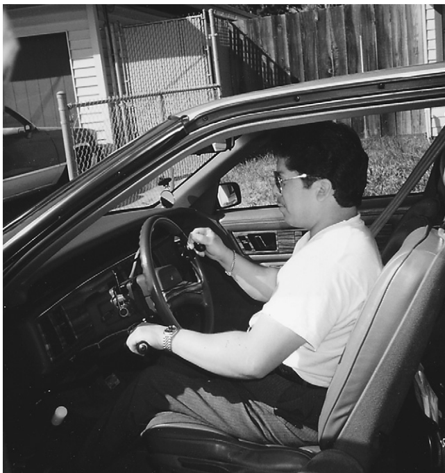
FIGURE 11-21 A basic setup for paraplegics includes spinner knob for steering and mechanical hand controls to operate accelerator and brake. This equipment can be used in many cars, vans, trucks, and sport utility vehicles.
