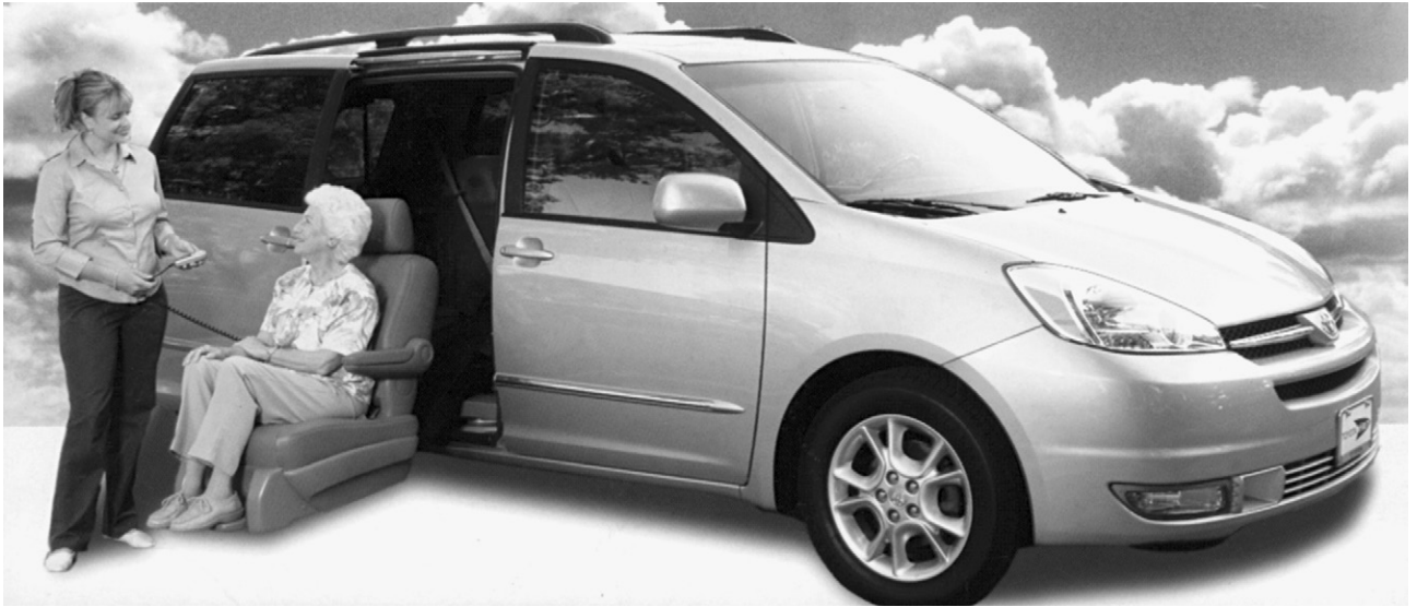
FIGURE 11-18 Bruno's Lift-Up power mobility seat for Toyota Sienna minivans aids vehicle entry by modifying activity demands for caregiver and client.
