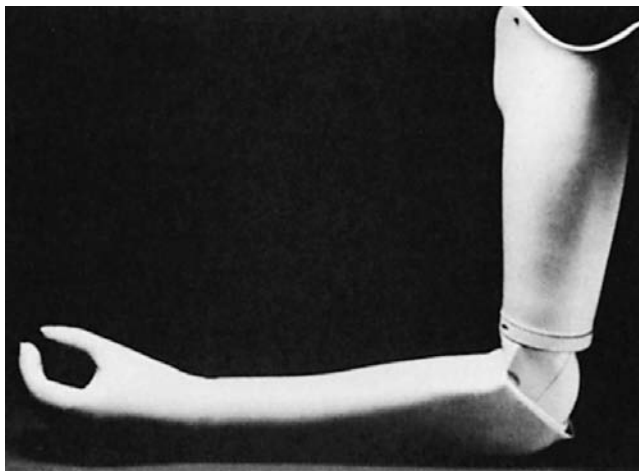
Figure 46-14 Utah arm with externally powered hand and elbow. (Photo courtesy of Motion Control, Salt Lake City, UT.)
