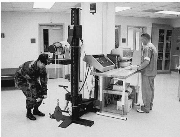
Figure 33-9 BTE Work Simulator used for dynamic strength testing.
