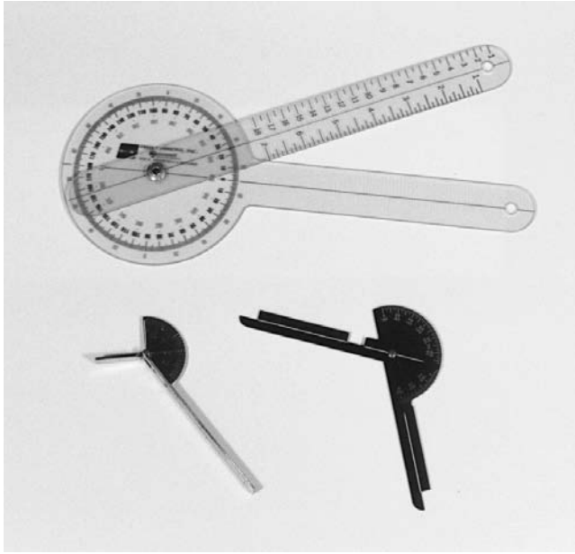
Figure 5-1 Three types of goniometers. The large full-circle goniometer ( top ) is used to measure large joints. The small finger goniometer ( bottom left ) has flat arms that fit over the fingers. The small half-circle goniometer ( bottom right ) is used to measure small joints, such as the wrist.
