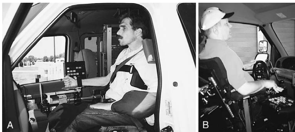
Figure 31-25 The Scott System allows many persons with polio, muscular dystrophy, C4–5 quadriplegia, and triplegia to drive independently. A. Person with C5 quadriplegia drives with the right hand in a tri-pin device. He pushes forward for gas and pulls back for braking, and supinates his forearm for turning right and pronates for turning left. B. One-handed steering with a small wheel by a person who uses his normal left extremity to push and pull the wheel for gas and brake; the wheel rotates 90° right or left for turning. (Courtesy of Driving Systems Inc., Van Nuys, CA.)
