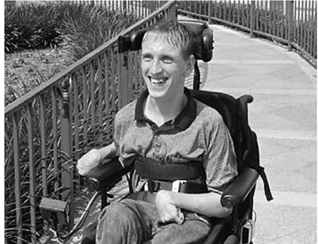
Figure 18-6 College student uses a power wheelchair controlled with proximity switches in a head array. The display in front of right armrest provides feedback regarding drive selection, environmental unit (ECU) functions, and battery level. A switch on the right side of the head array permits selection of drive and ECU functions. (Courtesy of Adaptive Switch Laboratories, Inc., Spicewood, TX.)
