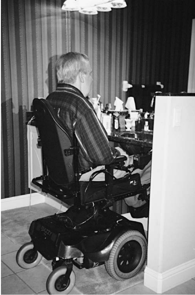
Figure 31-20 Use of a powered vertical up/down seat on a powered wheelchair to allow near approach to the sink for grooming.
