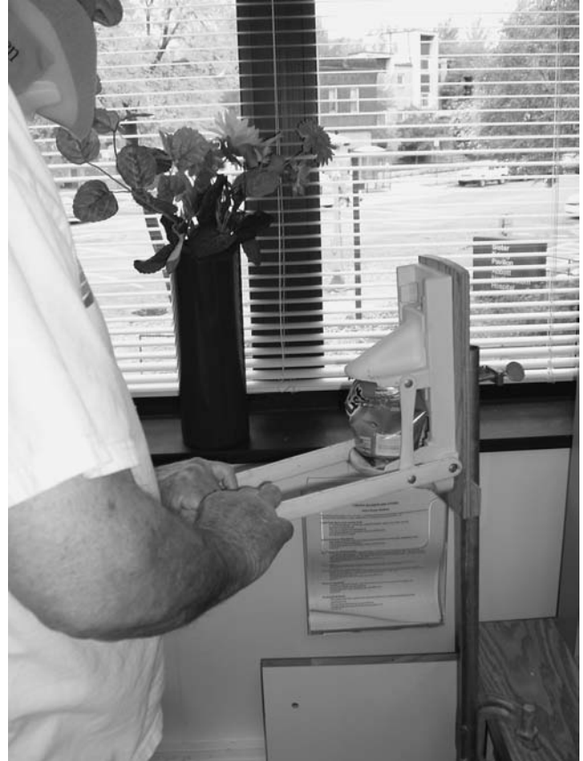
Figure 13-8 A patient who has weak upper extremities is able to crush cans for recycling because the handle (force arm) of the crusher has been elongated.
