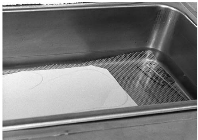
Figure 17-15 Heating the thermoplastic.
