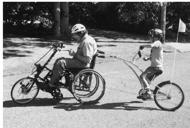
Figure 18-7 A father uses a cycling apparatus attached to his everyday-use manual wheelchair for outdoor activity with his children.
