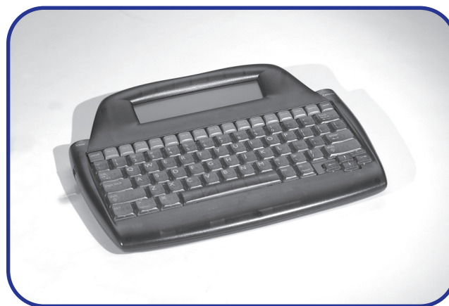
FIGURE 61.2 An AlphaSmart™ is an example of an inexpensive, portable word processor with adaptive features. It beams text to a computer, where it can be printed and saved.
