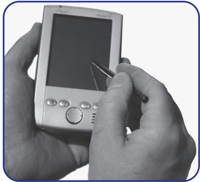
FIGURE 61.7 The PocketCompass™ offers pictures and stored speech as cognitive supports for sequencing activities. PDAs can also remind, report location, and support decisions.
