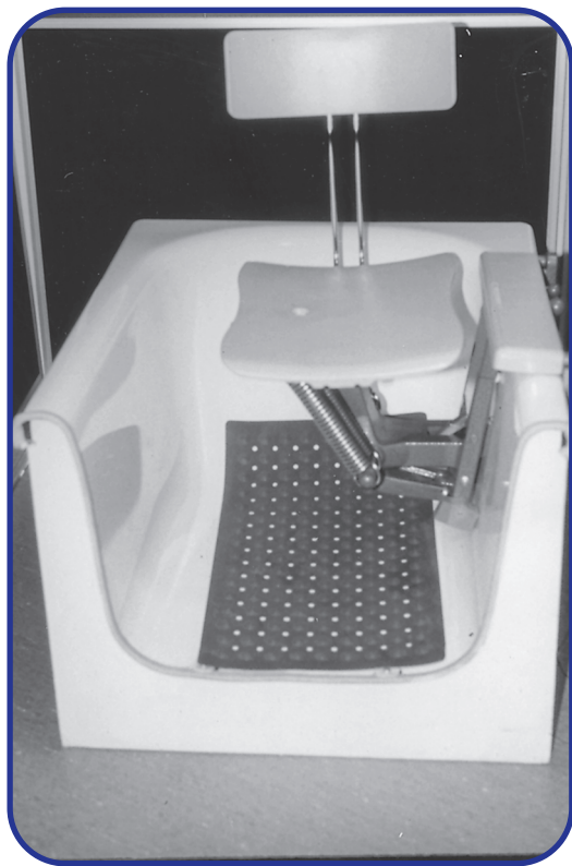
FIGURE 46.6 The mechanical tub seat is spring loaded and raises from the tub bottom with a weight shift and a simultaneous pushing up on the tub edges.
